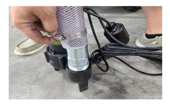
Attach other end of 2-inch braided hose to sump pump with hose clamp
