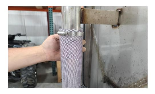
Attach one end of 2-inch braided hose to down spout on Ryedrator with hose clamp.
